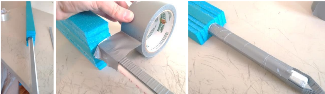
Figure 5.6 Placing the Duct Tape Strips
